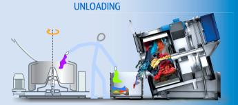
Forward tilting to ease unload after extraction.
